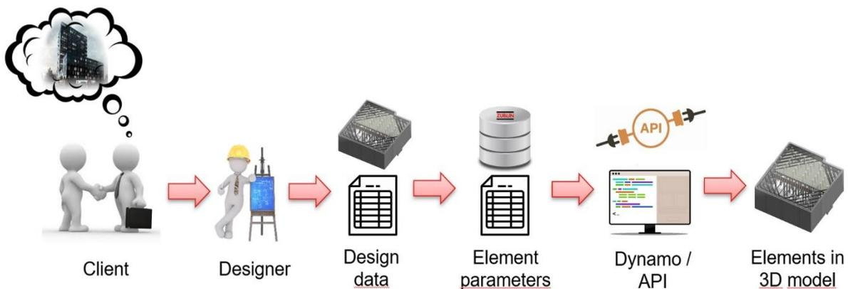
Figure 2: sequence of phases from concept to creation of Revit model by means of Dynamo scripts or Revit API.
