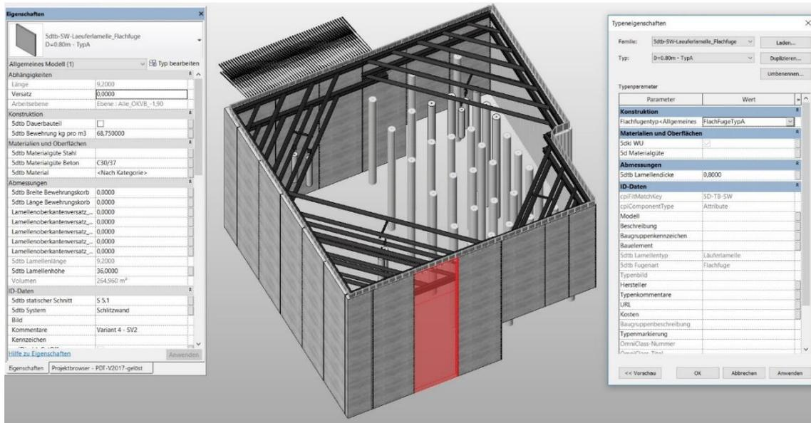
Figure 1: 3D visualization of a construction projects in Autodesk Revit together with its elements and related parameters.
