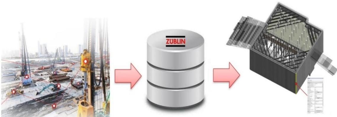
Figure 3: integration of production data from construction site to 3D model through database
